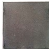
ZINCALUME® steel (No Sign of Rust)
